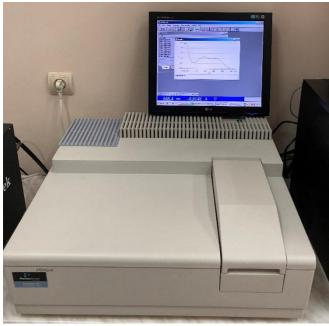
Double-beam scanning UV-Vis Spectrophotometer, PC operated via UVWinLab software (manufacturer Perkin Elmer, 2006).
