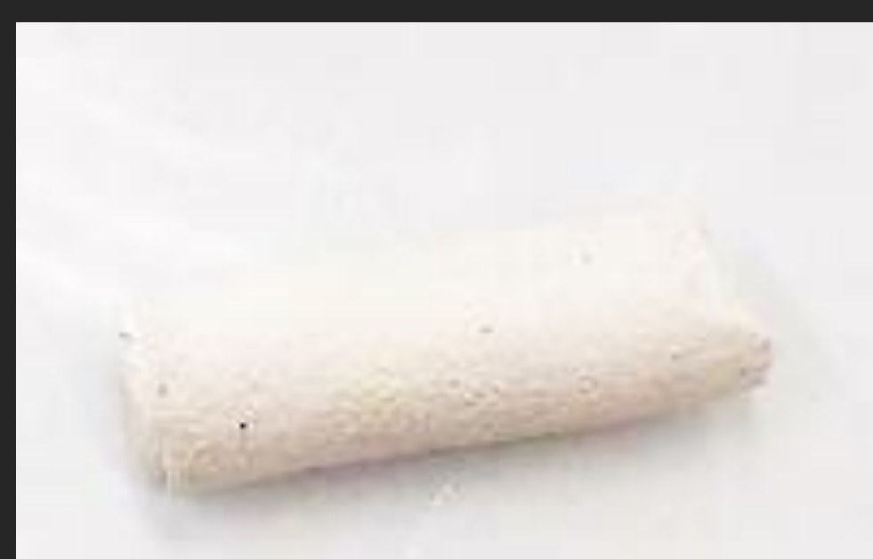
Fig. 1. Synthesized poly(HIPE) monolith.
