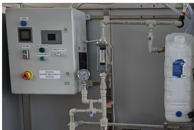
Fig. 1. flow-through laboratory non-thermal plasma system.
