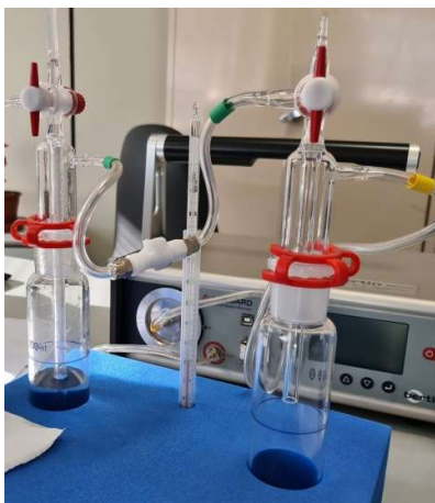
Fig. 1. Alphaguard DF2000 equipment to measure radon concentration in water samples.
